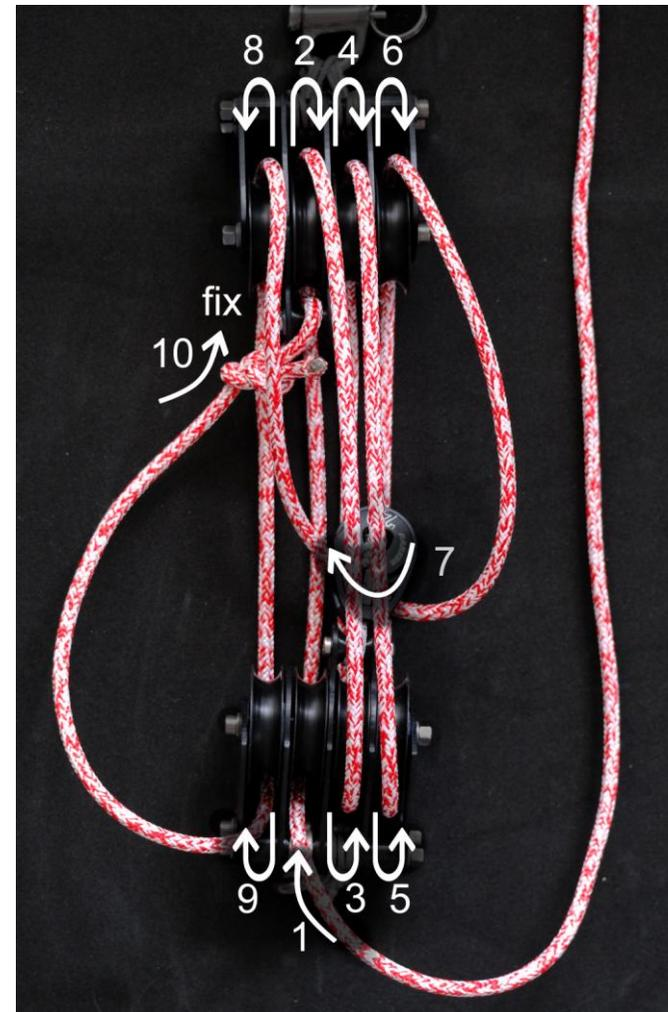
Attach one single block to bottom Quad Q-block, and ratchet to the clew of sail , that makes perfect 1:10 external mainsheet configuration for A Cat.
